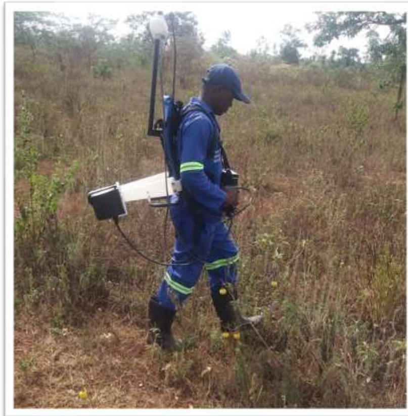
Figure 5 very low frequency ground magnetic surveys
