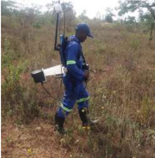
VLF Survey for sulphides in Ntungamo
